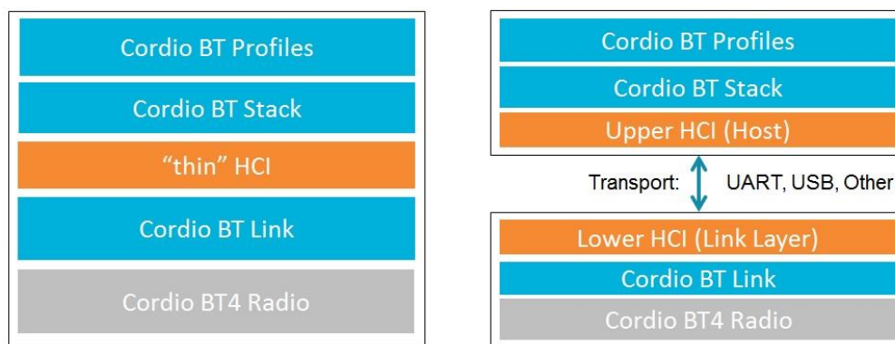
Figure 1. Cordio Stack and Profiles in a single-chip SoC system and dual-chip system
